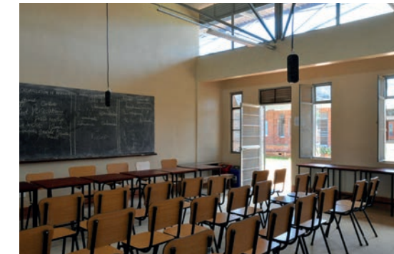
NTC Kairo Classrooms have light coloured walls to optimise daylighting and artificial lighting when in use
