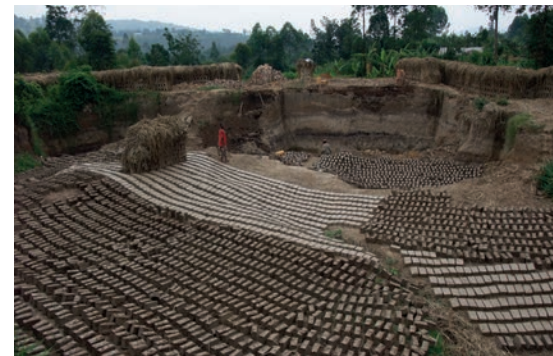
Lake Bunyonyi Secondary Bricks were moulded from good quality clay and sundried before being stacked up into giant furnaces
