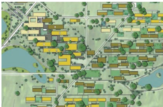
NTC Kaliro has a 3-phase masterplan, which orientates all new structures on an east-west axis
