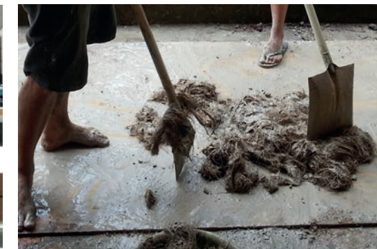
Possible materials for East African Biocrete: rice husks, ash from cassava peels, karroo gum and coconut fibres
